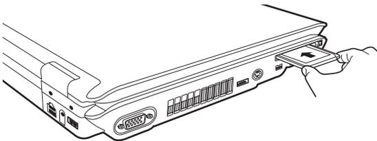
*(Sample Illustration) Inserting a PC Card*
