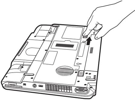
*(Sample Illustration) Unlocking the battery release lock*
