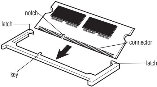
*(Sample Illustration) Aligning the memory module with the socket*
