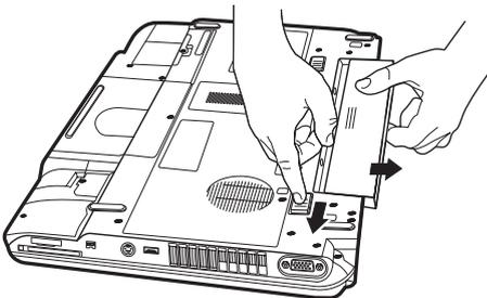
*(Sample Illustration) Removing the battery*
