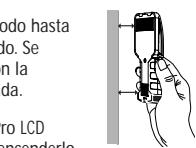
Without moving unit, squeeze and hold On/Off button. Wait for the beeping to stop and for the TruCal® icon to turn on.
