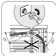
2. Connect the hose with the angled connection to the machine.
