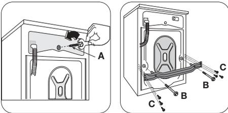
3. With a suitable spanner unscrew and remove the central rear bolt **A**.
