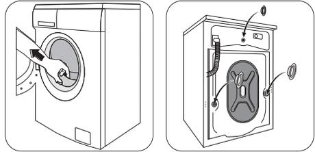
6. Open the porthole, take out the inlet hose from the drum and remove the polystyrene block fitted with the adhesive tape on the door seal. Open the porthole, take out the inlet hose from the drum and remove the polystyrene block fitted with the adhesive tape on the door seal.
