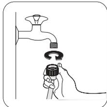
4. Connect the hose to a tap with a 3/4" thread. Always use the hose supplied with the appliance.
