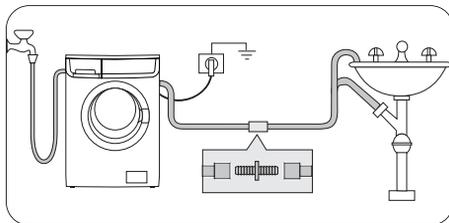
**In a sink drain pipe branch.** This branch must be above the trap so that the bend is at least 60 cm above the ground.
