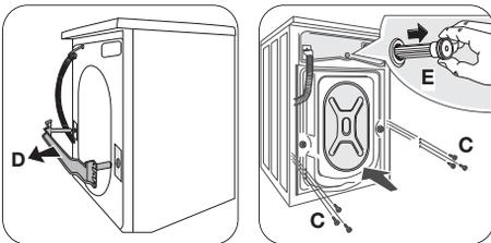
5. Remove the bracket **D**, refit the six smaller bolts **C** and slide out the relevant plastic spacer **E**.
