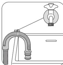
**Hooked over the edge of a sink using the plastic hose guide supplied with the machine.** In this case, make sure the end cannot come unhooked when the machine is emptying. This could be done by tying it to the tap with a piece of string or attaching it to the wall.
