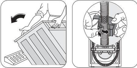
1. After removing all the packaging, carefully lay machine on it's back to remove the polystyrene base from the bottom.
