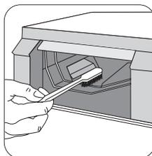
Having removed the drawer, use a small brush to clean the recess, ensuring that all washing powder residue is removed from the upper and lower
