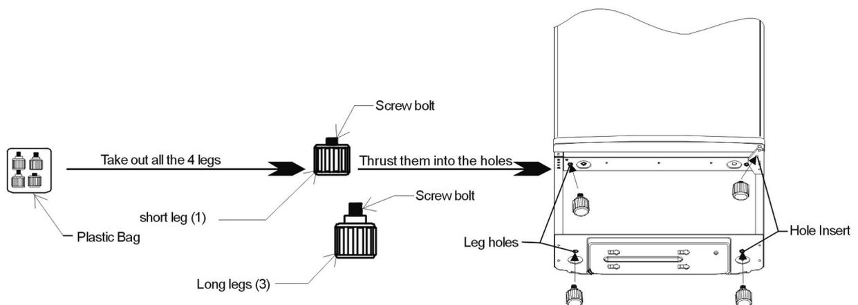
***Note :Must screw the short leg into the base bracket!***
