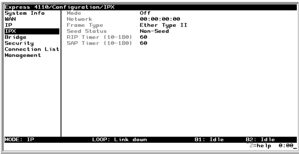
Figure 3-5. Configuration/IPX Screen
