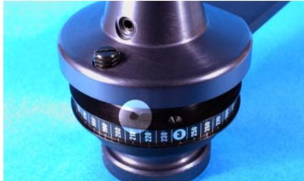
3) Depress the brass plunger and push up on the Indexing Ring until the brass plunger pops into the plunger hole and the pin slides into the notch.
