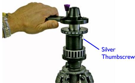
2) Once the thumbscrew is loosened, pull the Horizontal Bracket Assembly upward out of the Rotator Hub. You may need to wiggle it a bit as you lift it out of the hub.
