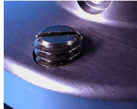
Be sure to not overtighten the plunger so that the metal body of the plunger would come in contact with the indexing ring. Also be sure that the plunger is not set deep enough as this will cause excessive play in the indexing action.
