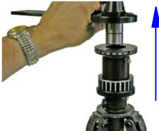
3) Once the Horizontal Bracket Assembly is removed, the Detent Disc can be changed by grabbing the protruding tab on the detent ring and pulling it up out of the Rotator Housing.
