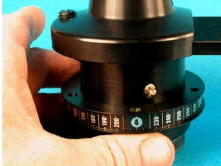
2) Rotate the Indexing Ring to line up the notch on the top of the Indexing Ring with the black slanted alignment pin at the top of the Rotator Base. The pin will eventually go into the notch.
