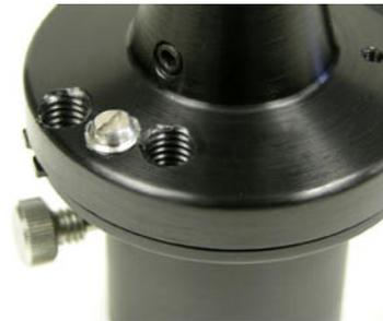
Be sure to not overtighten the plunger so that the metal body of the plunger would come in contact with the indexing ring. Also be sure that the plunger is not set deep enough as this will cause excessive play in the indexing action.
