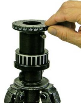
4) The new Detent Disc is installed by pushing it into the recessed area in the top of the Rotator Hub as shown at left.
