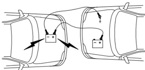
4. Make the final connection of the negative (-) cable to an exposed metal part of the stalled vehicle's engine, away from the battery and the carburetor.
