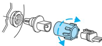
6. Without turning, remove the old bulb from the lamp assembly by gently pulling it straight out of the lamp assembly.
