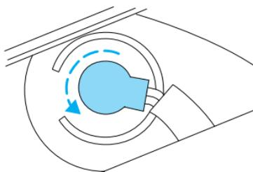
2. Pull the bulb straight out of the socket and push in the new bulb.
