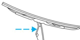
2. Turn the blade at an angle from the wiper arm. Push the lock pin manually to release the blade and pull the wiper blade down toward the windshield to remove it from the arm.
