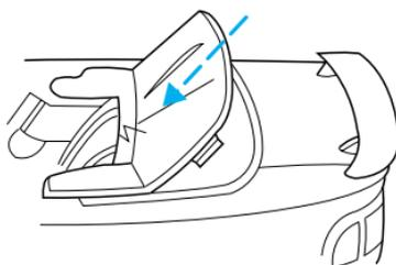
2. Push boot forward until rear attachment engages under molding.
