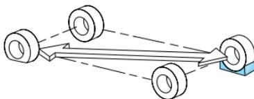
2. Place gearshift lever in P (Park) or R (manual transmission), turn engine OFF, and block the diagonally opposite wheel.
