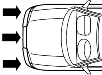
The fact that the air bags did not inflate in a collision does not mean that something is wrong with the system. Rather, it means the forces were not of the type sufficient to cause activation. Air bags are designed to inflate in frontal and near-frontal collisions, not rollover, side-impact, or rear-impacts.
