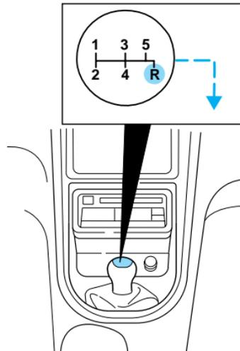
**If R (Reverse) is not engaged, continue to push the clutch pedal in while you put the**
