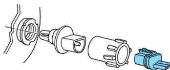
5. Remove the bulb retaining ring by rotating it counterclockwise (when viewed from the rear) about  $\frac{1}{4}$  turn to free it from the bulb socket, and slide the ring off the plastic base. Keep the ring to retain the new bulb.
