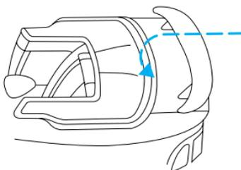
3. Push forward flap of boot until both clips engage under trim panel edge. Repeat on other side of vehicle.
