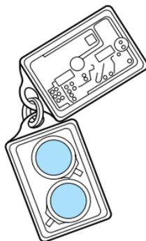
2. Place the positive (+) side of new batteries down. Refer to the diagram inside the transmitter unit.
