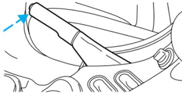
Push the button on the end of the parking brake and push the handle down as far as possible to release the brake. Driving with the parking brake on will cause the brakes to wear out quickly and reduce fuel economy.
