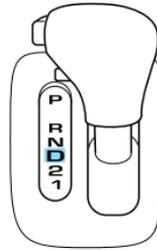
**D (Overdrive)** can be deactivated by pressing the transmission control switch on the end of the gearshift lever.
