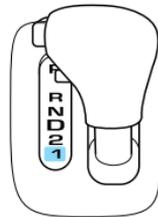
Selecting 1 (Low) at higher speeds causes the transmission to shift to a lower gear, and will shift to 1 (Low) after vehicle decelerates to the proper speed.
