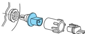
need to turn the bulb left or right to align the grooves in the plastic base with the tabs in the lamp assembly. When the grooves are aligned, push the bulb into the lamp assembly until the plastic base contacts the rear of the lamp assembly.
