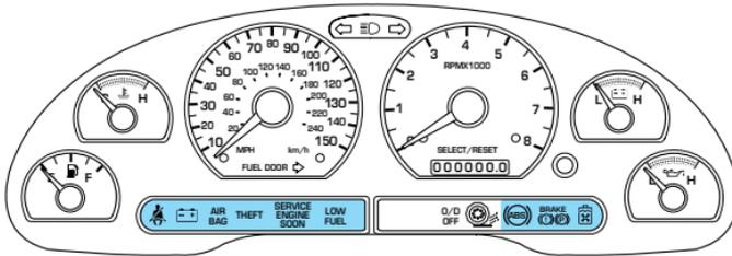
Make sure the corresponding lights illuminate briefly. If a light fails to illuminate, have the vehicle serviced.
