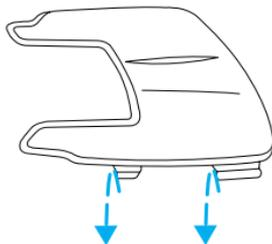
5. Push and pull front of boot to ensure tongue is engaged into groove.
