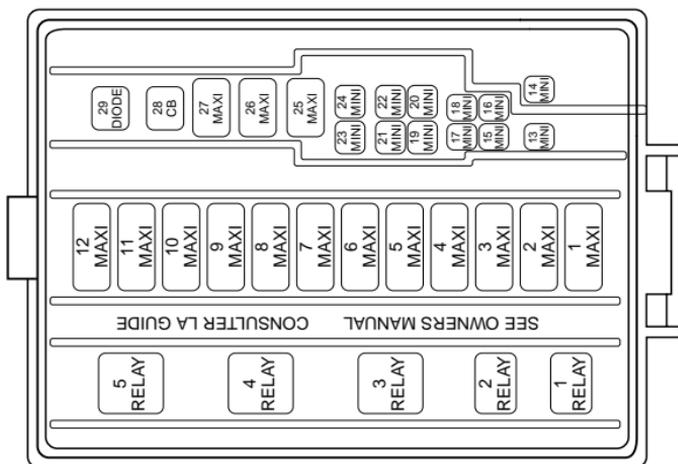
The high-current fuses are coded as follows.
