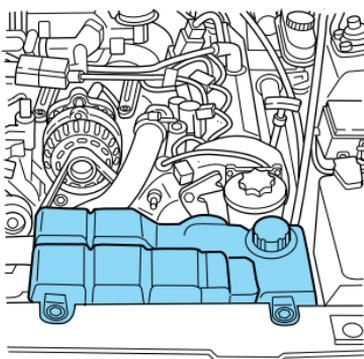
Check the level of the engine coolant in the reservoir. Refer to the Scheduled Maintenance Guide for service interval schedules. Be sure to read and understand *Precautions when servicing your vehicle* in this chapter.
