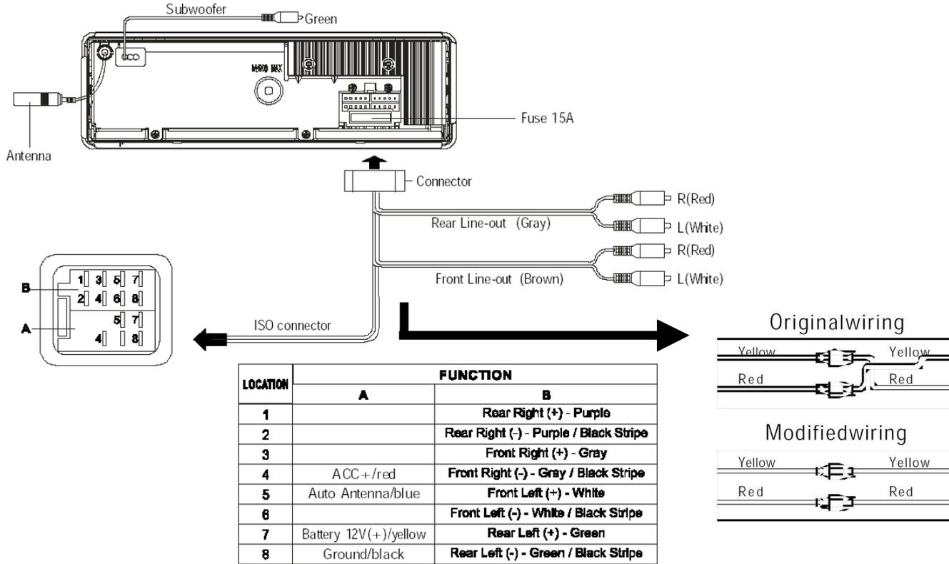
Do not interchange the connection of the wiring!!!
