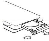
2. Insert the button-type battery with the stamped(+) mark facing upward.
