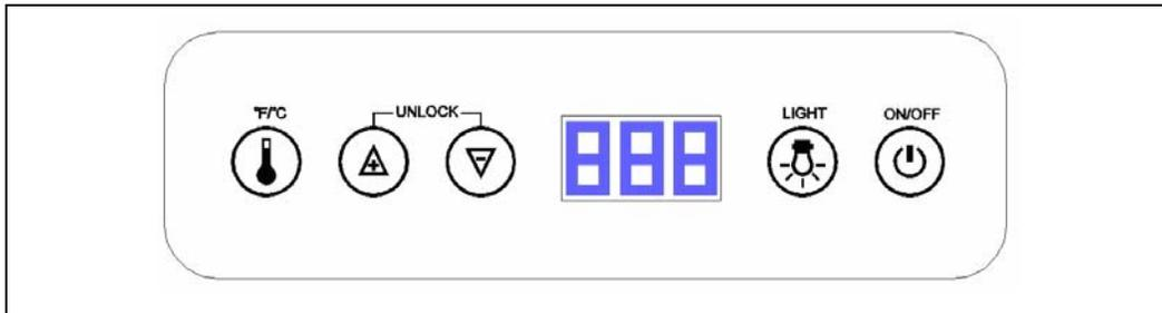
You can select temperature display setting from Fahrenheit to Celsius degree by pushing the °F/°C button/mark. Fahrenheit or Celsius degrees indicator will appear in blue color in the temperature display window.
