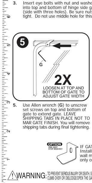
Use Allen wrench (G) to unscrew set screws on top and bottom of gate to extend gate. LEAVE SHIPPING TABS IN PLACE NOT TO MAR GATE FINISH. You will remove shipping tabs during final tightening.
