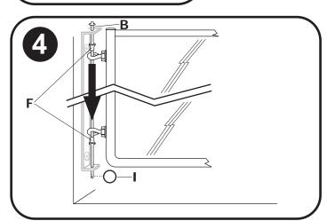
Hang gate by inserting hinge rod  $(\mathbf{B})$ , through top of mounted hinge bracket  $(\mathbf{A})$ , through upper plastic 4. shoulder washer (F), through both eye bolts, through lower plastic shoulder washer (F), and finally through bottom of hinge bracket. To secure hinge, insert key ring (I) through hole in end of hinge rod.
