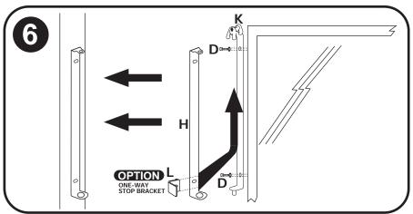
Mount latch assembly (K) to gate using 3/4" bolts with serrated washers (**D**). Attach wall mount for latch assembly (**H**) up into part (**K**) that is now secure on gate. Slide gate out to mark holes for (**K**) on attaching wall. (\*OPTIONAL ONE WAY BRACKET INSTALLED HERE) Then attach the wall mount of latch assembly to wall using Phillips head screws (C).
