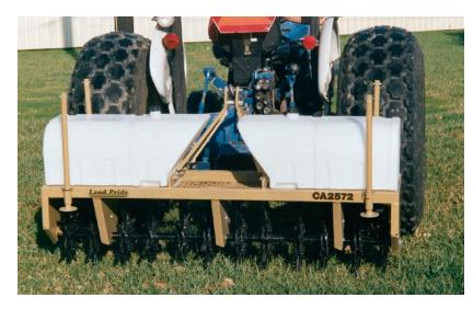
Optional Water Tanks are available on the 60" and 72" Core Aerators for additional weight to aid in spoon penetration. Water drains easily from the tanks through the bottom drain holes, reducing weight to the desired amount.
