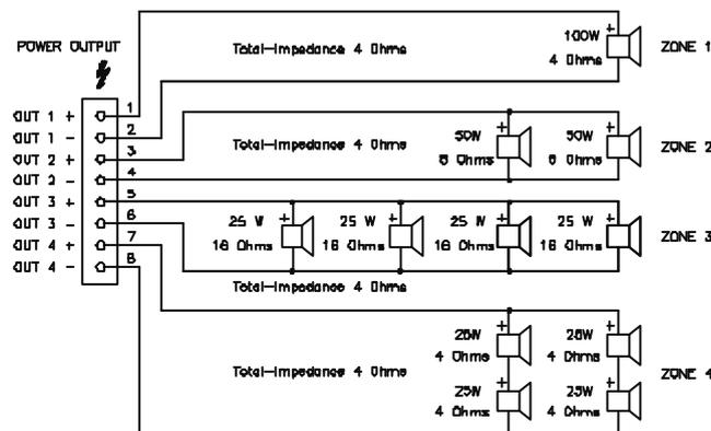
diagram 4 Connection of low-impedance loudspeaker systems
