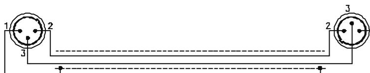
diagram 2 LF-cable for coupled operation of two DPA 4411
