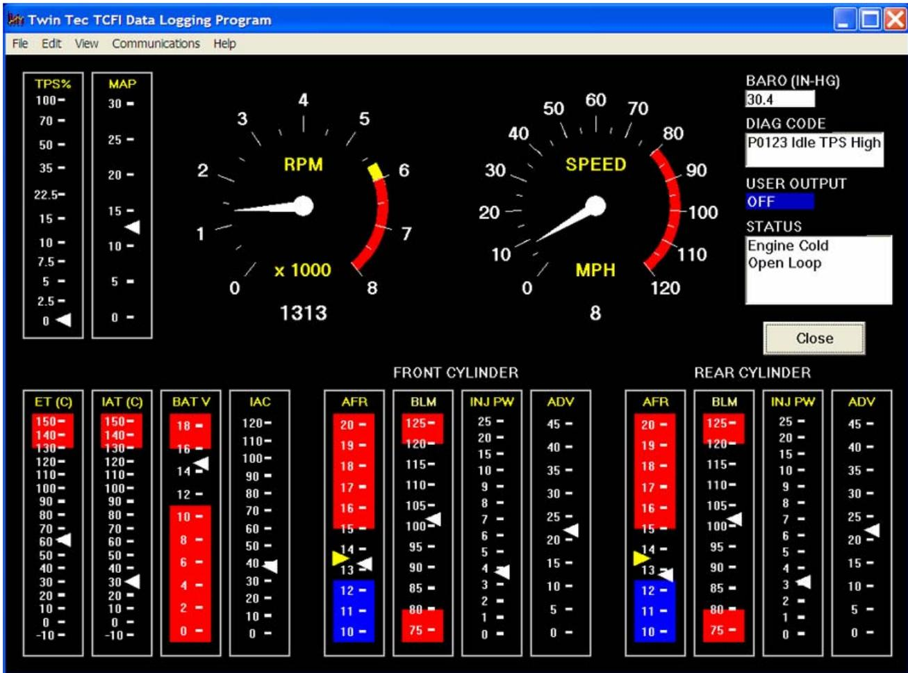
**AFR** – the air/fuel ratio bar graph has dual pointers. The yellow pointer on the left side is the air/fuel ratio command (from AFR table). The white pointer on the right side is the actual air/fuel ratio based on the exhaust gas oxygen sensor reading. Note that the value will remain near 10 until the sensor has warmed up. Front and rear cylinder AFR values are displayed for TCFI IID units.
