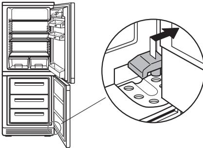
3. Wash the inside of the appliance with lukewarm water with a little bicarbonate of soda added (5 ml to 0.5 litre of water). Do not use soap or detergent as the smell may linger. Dry the appliance thoroughly. Remove the transport fittings from the storage shelves:
