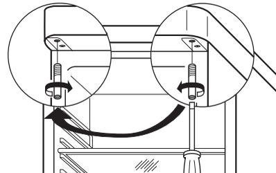
9. Move the door handles from the left to the right and cover the remaining holes with the hole cover pins.
