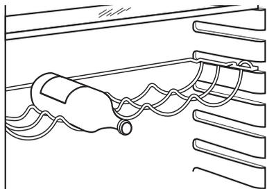
1. To do this pull the bottle rack forward until it can be tilted upwards, then slide the front support into the next level up.
