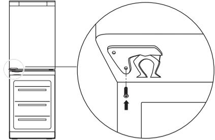
11. Carefully slide the fridge compartment door onto the top bearing pivot and close.
