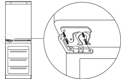
**13.** Fasten the self-closing mechanism on the top left of the freezer compartment door,
