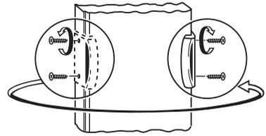
10. Fasten the self-closing mechanism to the bottom left of the fridge compartment door.
