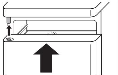
12. Slide the centre door bearing into the bottom left of the fridge compartment door and fasten to the housing.
