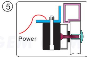
5 Turn on the power of EM-Lock, and let the armature plate bonds to the EM-lock. Adjust the position between the L bracket and the door frame.
