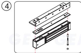
4 Lock the armature plate and L bracket first. Put the electromagnet into the armature plate second.
