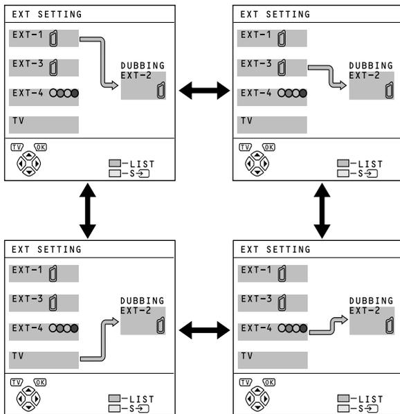
The arrow in the menu represents a signal flow. The left side of the arrow shows a signal source output from the EXT-2 terminal.
