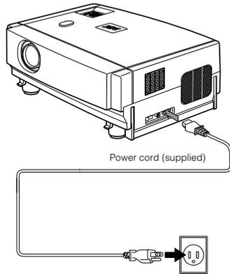
**1** Insert the supplied power cord into the power input terminal of the projector.
