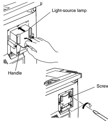
**4 Replace the lamp-replacement opening cover and fasten the screws.**
