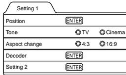
Decoder is only displayed when there is a signal for the Video IN terminal.
