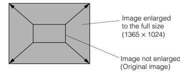
**Aspect:** While maintaining the original aspect ratio, the video image projected is virtually enlarged until either the horizontal or vertical side reaches the full size (1365 pixels × 1024 pixels).
