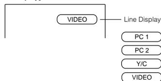
\* To show the line display (Y/C, VIDEO, PC1, or PC2) or not is selectable by the menu. Refer to "Setting and Adjusting Other Functions (OPTIONS)" on page 52.
