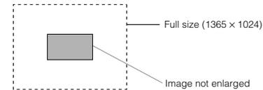
**Panel:** The picture image projected is virtually enlarged to the full size (1365 pixels × 1024 pixels). The horizontal and vertical enlargement ratio will differ depending on the original image and the image will be deformed.
