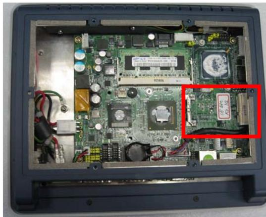
2. The socket latches are clipped on to the edges of the Mini card socket. Install wireless LAN card to the socket.
