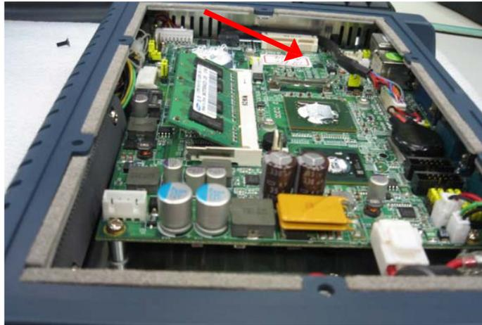
4. Install the memory module into the socket and push it firmly down until it is fully seated. The socket latches are levered upwards and clipped on to the edges of the SO-DIMM socket.
