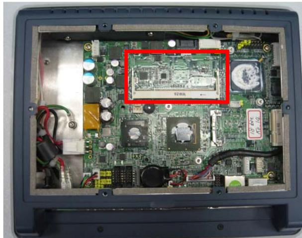
3. Push down latches on each side of the SO-DIMM socket.
