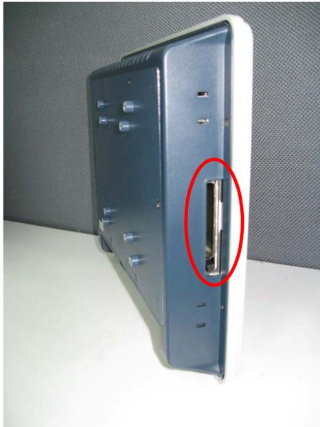
**Step 3** Locate the CompactFlash™ socket, and insert the card into the socket.
