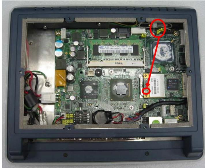
4. There are two connectors on wireless LAN card. One is MAIN, and the other is auxiliary. Connect antenna cable to **MAIN** connector on wireless LAN card.
