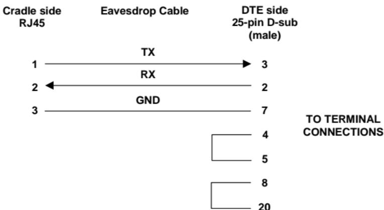
The **black flat** cable allowing the Modem connection has the following pinout:
