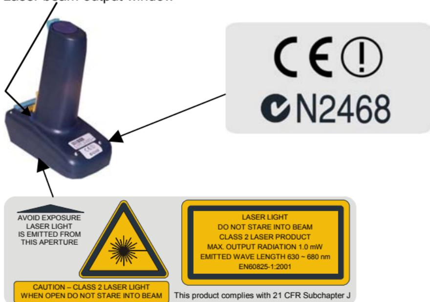
Figure 2 - F725-E/RF Laser Safety Labels
