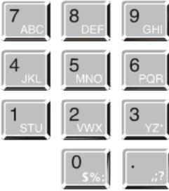
**NUMERIC AND ALPHANUMERIC KEYS:** allow the entry and display of the main numeric symbol. If the <SHIFT> has first been pressed, the choice of alternative alphabetic characters will be activated.
