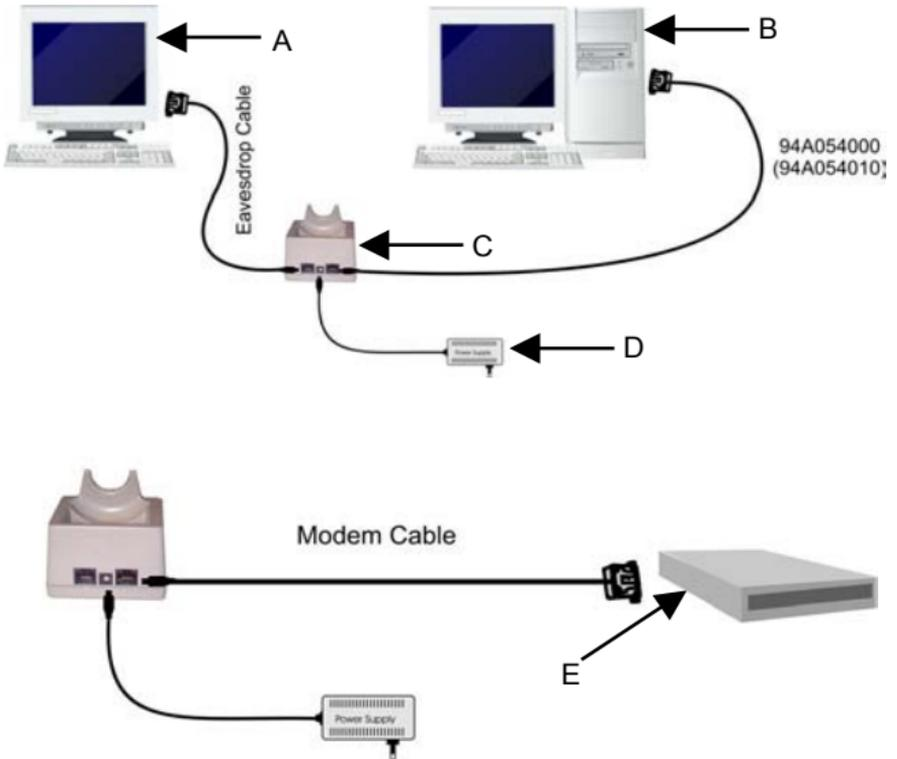
Figure 9 - Eavesdrop and Modem Connection
