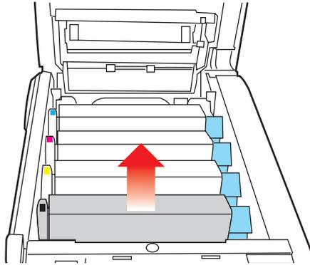
4. Put the assembly down gently onto a piece of paper to prevent toner from marking your furniture and to avoid damaging the green drum surface.
