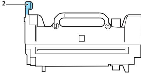
7. Lower the fuser into the printer.
