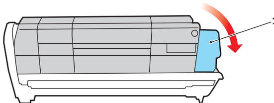
6. Lift the right-hand end of the cartridge and then draw the cartridge to the right to release the left-hand end as shown, and withdraw the toner cartridge out of the image drum cartridge. Place the cartridge on a piece of paper to avoid marking your furniture.
