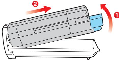
7. Take the new image drum cartridge out of its packaging and place it on the piece of paper where the old cartridge was placed. Keep it the same way round as the old unit. Pack the old cartridge inside the packaging material for disposal.
