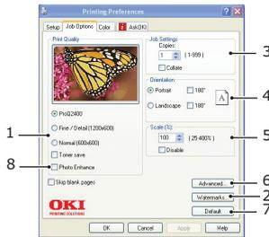
1. The output resolution of the printed page can be set as follows.
