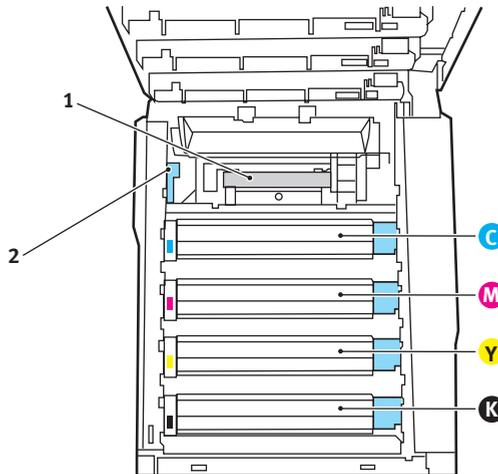
3. Pull the fuser retaining lever (2) towards the front of the printer so that it is fully upright.
