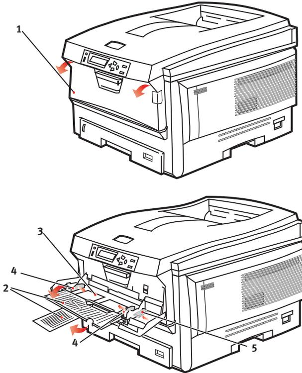
3. Press gently down on the paper platform (3) to ensure it is latched down.
