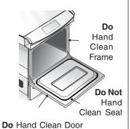
To clean oven door, wash with hot, soapy water and a clean cloth. DO NOT immerse the door in water.
