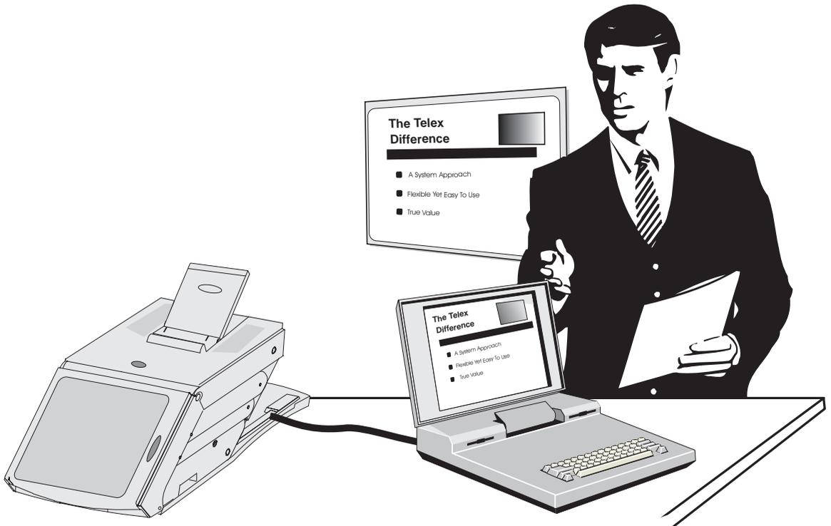
The Firefly™ P350 can be connected to any IBM or IBM compatible computer equipped with a VGA/SVGA video output. The P350 can also be connected to any Apple Macintosh computer that is equipped with a standard Macintosh video output.
