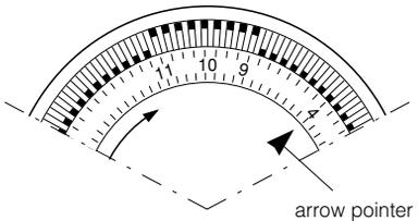
**Note:** Never turn the dial in an anti-clockwise direction!
