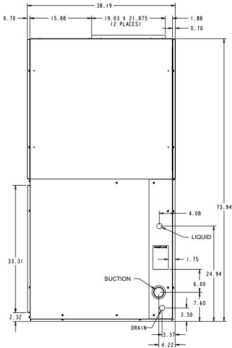
FIGURE 20 - LA300 PIPING CONNECTIONS
