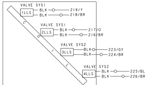
FIGURE 19 - 30, 40 & 50 TON LIQUID LINE SOLENOID WIRING
