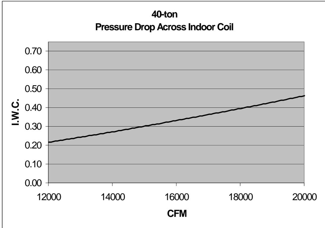
FIGURE 28 - 40 TON - PRESSURE DROP VS. CFM ACROSS INDOOR COIL (DOMESTIC)
