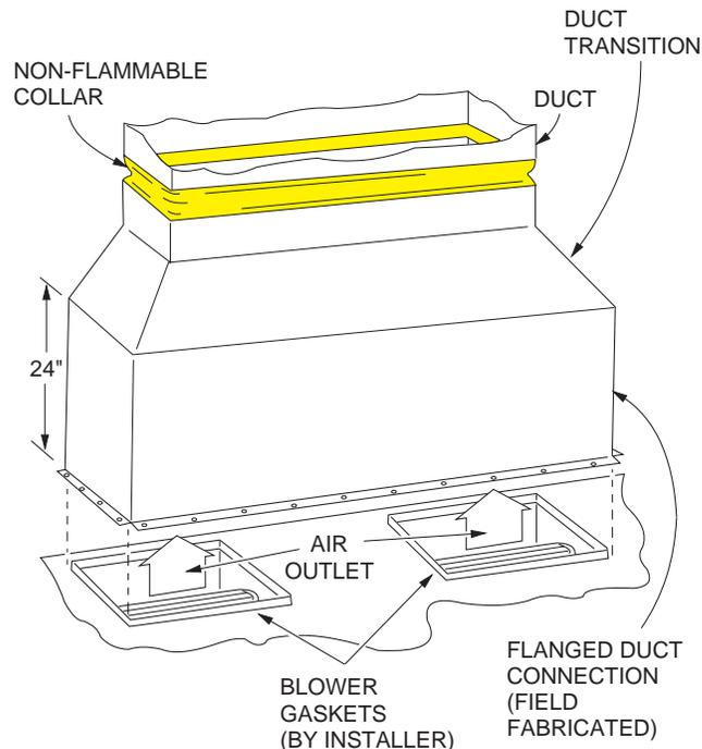
**FIGURE 13 - SUGGESTED METHOD FOR CONNECTING DUCTWORK**
