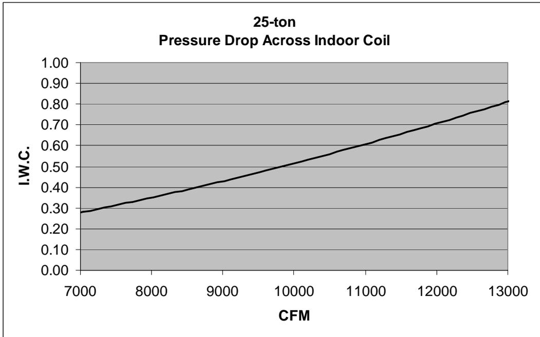
**FIGURE 26 - 25-TON PRESSURE DROP VS. CFM ACROSS INDOOR COIL**
