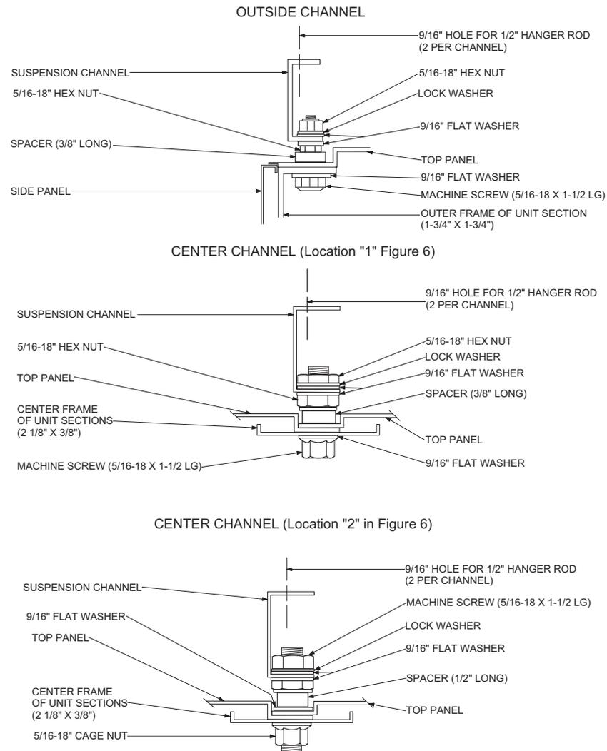
**FIGURE 12 - DETAILS FOR SECURING SUSPENSION CHANNELS**
