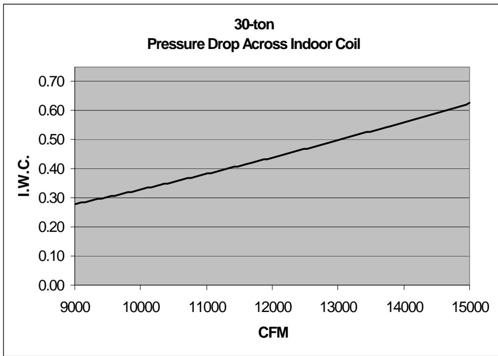
**FIGURE 27 - 30-TON - PRESSURE DROP VS. CFM ACROSS INDOOR COIL**
