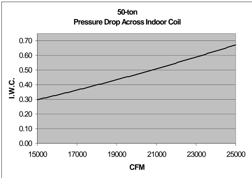
FIGURE 29 - 50 TON - PRESSURE DROP VS. CFM ACROSS INDOOR COIL
