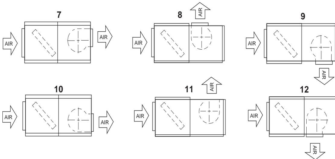
**FIGURE 7 - HORIZONTAL AIRFLOW ARRANGEMENTS**
