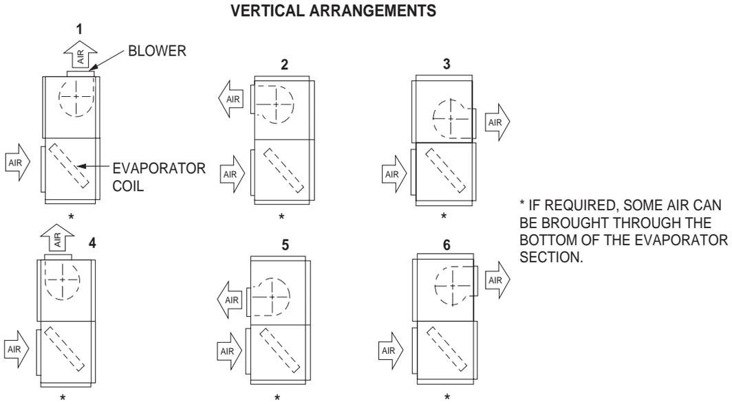
**FIGURE 6 - VERTICAL AIRFLOW ARRANGEMENTS**
