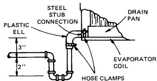
**FIGURE 14 - RECOMMENDED DRAIN PIPING
