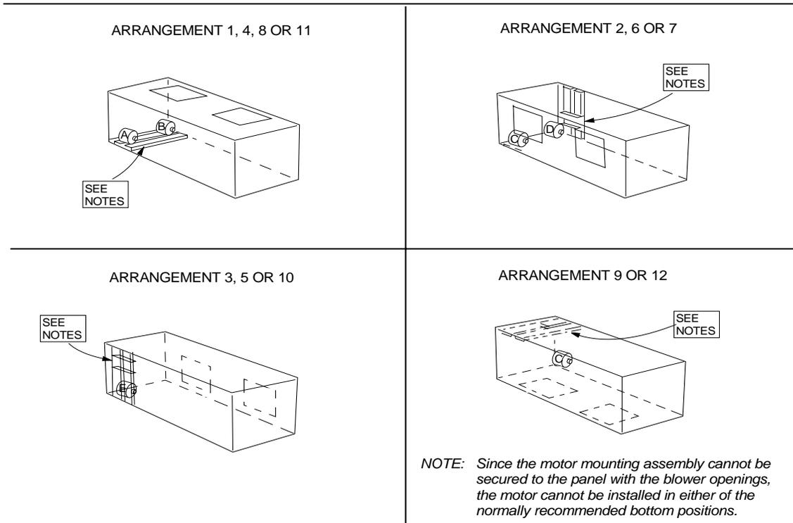
**FIGURE 5 - LA300/LB360/LB480 MOTOR ARRANGEMENTS**
