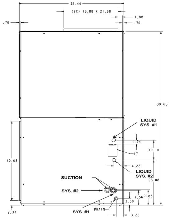
FIGURE 22 - LB480 PIPING CONNECTIONS
