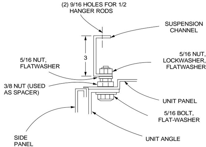
**FIGURE 9 - DETAILS FOR SECURING BOTTOM MOUNTING SUPPORTS**
