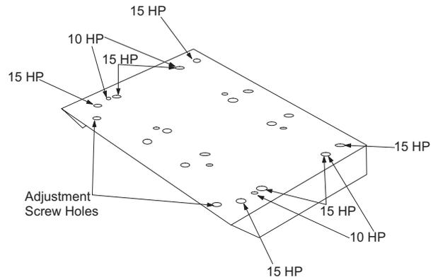
**FIGURE 3 - LB600 MOTOR MOUNT PLATE**
