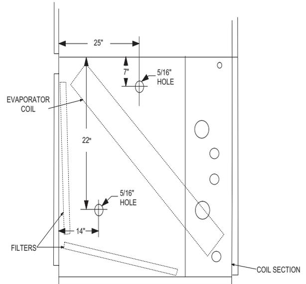
**FIGURE 25 - HOLE LOCATION FOR PRESSURE DROP READING**
