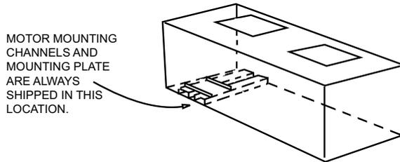
**FIGURE 1 - LA300 AN LB360/LB480 FACTORY MOTOR MOUNTING POSITION**
