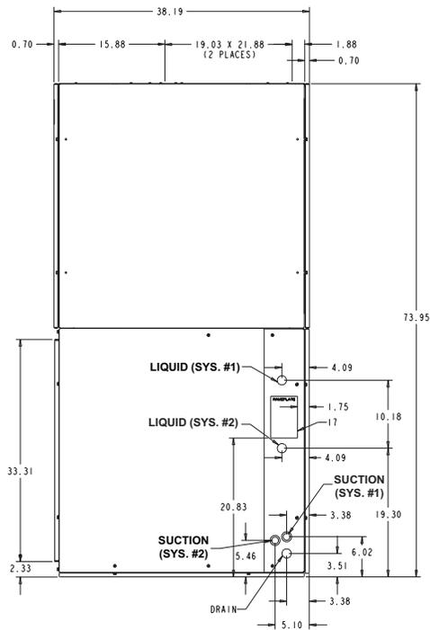
FIGURE 21 - LB360 PIPING CONNECTIONS
