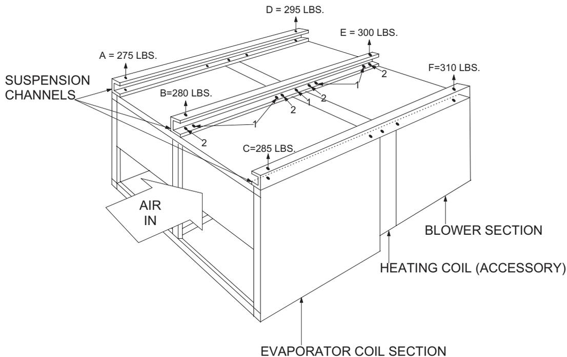
**FIGURE 11 - LB600 WEIGHT DISTRIBUTION WITH SUSPENSION APPLICATION**
