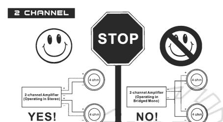
Two 4-ohm speakers, wired in stereo, will present a 4 ohm load to each channel of the amplifier. Most two-channel amplifiers will work well in this configuration.
