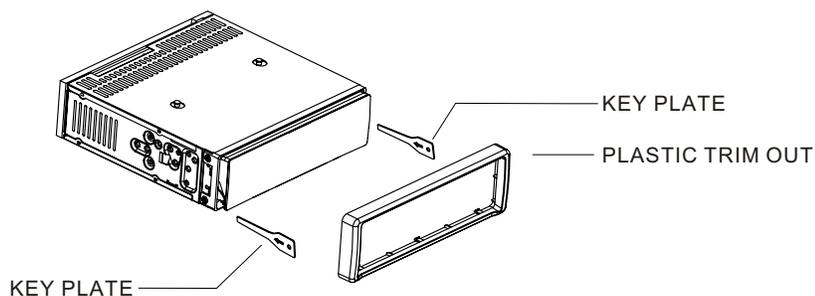
1. WHILE INSTALLING THE FRONT PANEL, PLEASE MOUNT THE LEFT SIDE FIRST, AND MAKE THE DIRECTION HOLE ON THE FRONT PANEL AIM AT THE LEFT GUIDE ON THE UNIT
