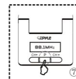
7. To keep regular used frequency in memory, please set it as current frequency. Press down P for seconds until CH NO flashes to enter CH saving mode. Adjust CH+, CH- to choose the location(CH NO.) for the frequency you want to save. Press P to keep both CH NO and frequency in memory.
