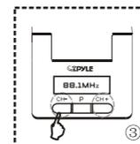
3. Press frequency up/down to set a suitable one for using. LCD display shows the frequency in using.
