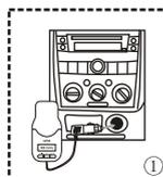
1. Plug cigar head into car cigarette lighter socket. LCD display lights up and shows current frequency.
