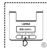
6. Press "P" to select previous stored channel. The frequency will cycle from CH01 to CH10. LCD will display first the selected CH NO and then frequency after one second.
