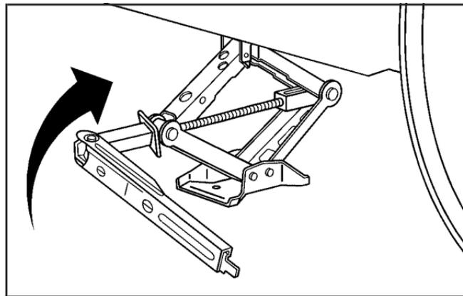
3. Raise the vehicle by turning the jack handle clockwise. Raise the vehicle far enough off the ground so there is enough room for the compact spare tire to fit underneath the wheel well.
