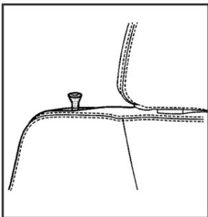
5. Pull up on the knob located on the top of the seatback on the outboard side to release the seatback. With your other hand, pull the seatback forward.
