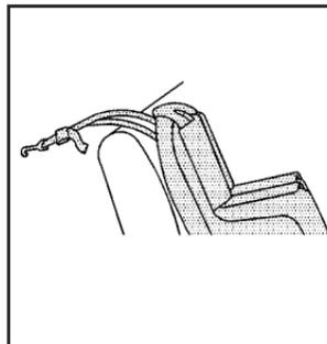
If the position you are using does not have a head restraint and you are using a dual tether, route the tether over the seatback.
