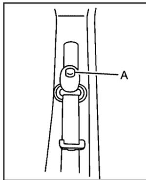
To move it down, press the release button (A) and move the height adjuster to the desired position. You can move the height adjuster up just by pushing up on the shoulder belt guide.
