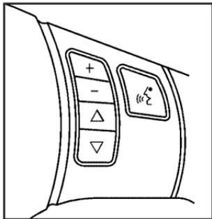
Radio controls are located on the right side of the steering wheel. If your vehicle has this feature, some audio controls can be adjusted at this location. They include the following:
