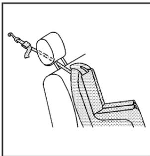
If the position you are using has a fixed or adjustable head restraint and you are using a single tether, route the tether under the head restraint and in between the head restraint posts.
