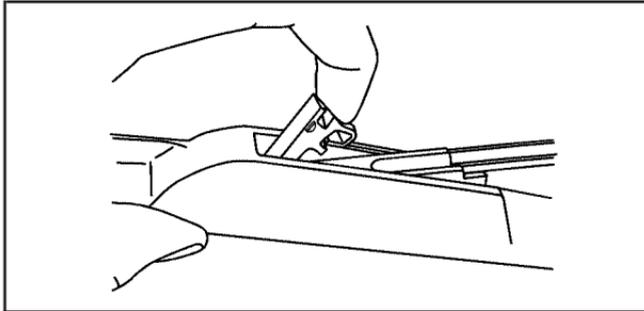
2. While holding the wiper arm, lift the clip up from the blade connecting point, and pull the blade assembly down toward the windshield to remove it from the wiper arm.
