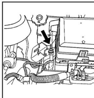
The remote positive terminal is located under a red tethered cap on the engine compartment fuse block. Remove the cap to access the terminal.
