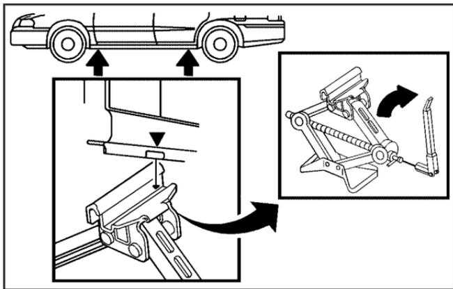
2. Position the jack and raise the jack lift head to fit over the car flange under the down arrow markings on the rocker panel.
