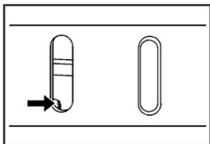
2. Locate the release lever on the latch.
