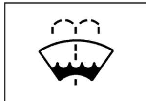
Open the cap with the washer symbol on it. Add washer fluid until the tank is full. See *Engine Compartment Overview on page 298* for reservoir location.
