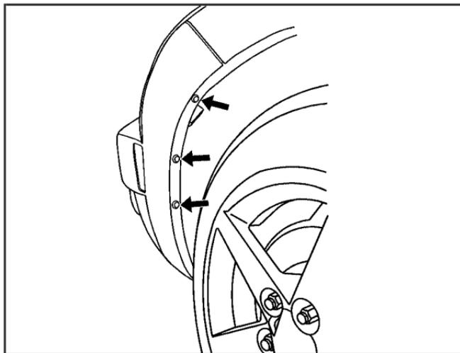
2. Remove the fasteners to access the headlamp and the turn signal/parking lamp bulbs.
