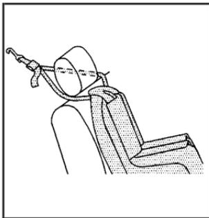
If the position you are using has a fixed or adjustable head restraint and you are using a dual tether, route the tether around the head restraint.
