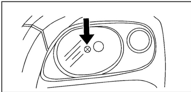
2. Find the aim dot on the lens of the low-beam headlamp.
