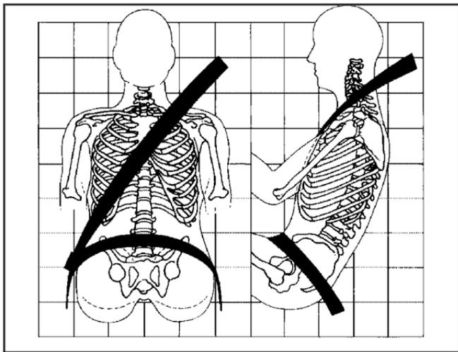
The lap part of the belt should be worn low and snug on the hips, just touching the thighs. In a crash, this applies force to the strong pelvic bones. And you would be less likely to slide under the lap belt. If you slid under it, the belt would apply force at your abdomen. This could cause serious or even fatal injuries.
