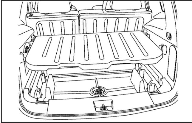
The third position is with the front corners placed in the lower guides and the rear corners placed in the upper guides. Do not load cargo on the panel in this position. The fourth position is with the front corners placed in the lower guides closest to the rear seat for subfloor access. Do not drive while the panel is in this position.
