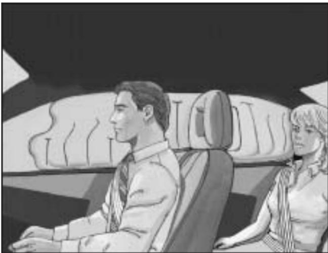
If your vehicle has a roof-mounted side impact airbag for the right front passenger and the person directly behind that passenger, it is located in the ceiling above the side windows.
