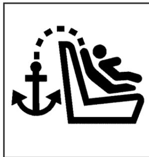
To assist you in locating the top tether anchors for the rear seats, the top tether anchor symbol is located on the storage compartment and the cargo mat behind the rear seats.
