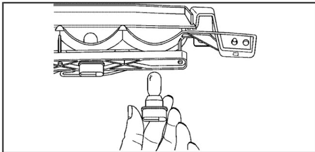
6. Pull the bulb straight out of the socket.
