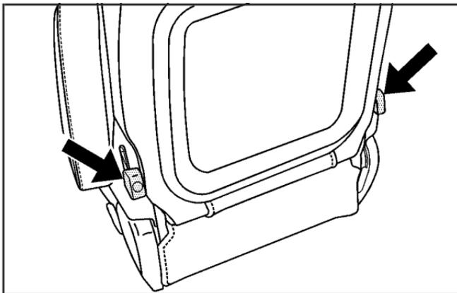
3. Use one of two levers to fold the seat flat. The levers are located on the rear of the seat near the bottom of either side of the seat. Pull up on either lever and fold the seat forward until the seatback disengages. This can most easily be done from the rear seats.
