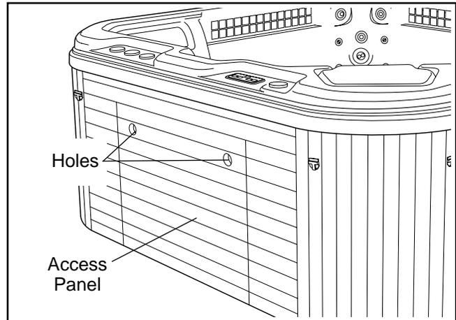
To replace the access panel, insert the bottom of the access panel into the lip of the spa base. Push the access cover in until it is securely in place.
