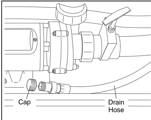
5. When the spa is empty, close the valve and remove the garden hose. Re-attach the cap and return the drain hose inside the spa.
