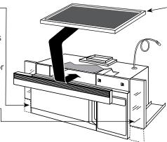
Filter kits JX81A– Recirculating Charcoal Filter kit To be used when the Spacemaker microwave oven cannot be vented to the outside.
