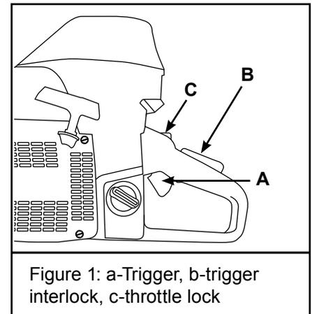
Figure 1: a-Trigger, b-trigger interlock, c-throttle lock
