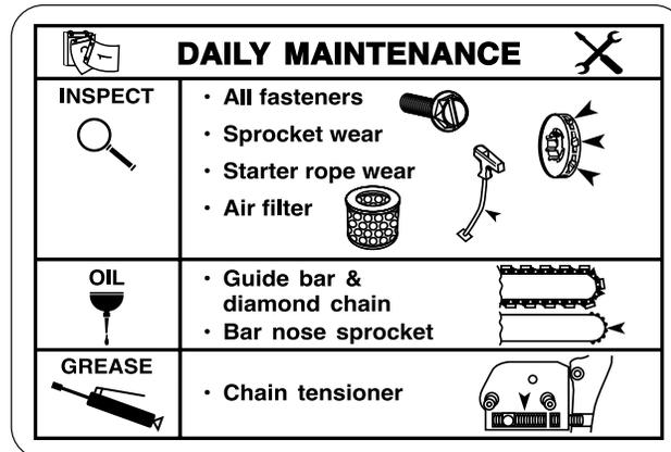
3. Inspect and tighten all fasteners as necessary.
