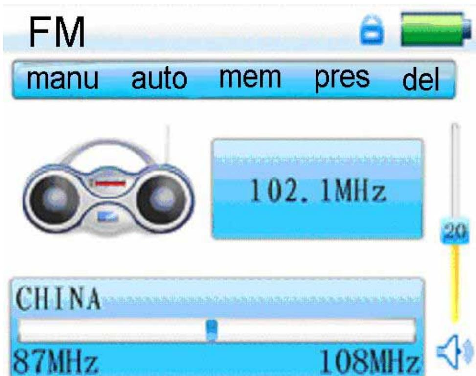
Manu: Press MENU Key to confirm, press left or right to change the frequency manually, long press the [MENU] key to exit.
