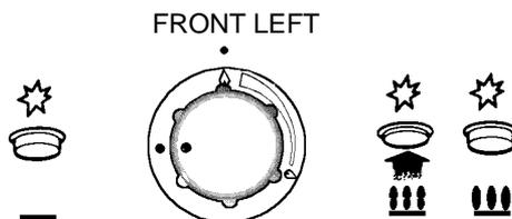
Warning: If the ignition button is not pressed immediately a build up of gas may cause the flame to spread.
