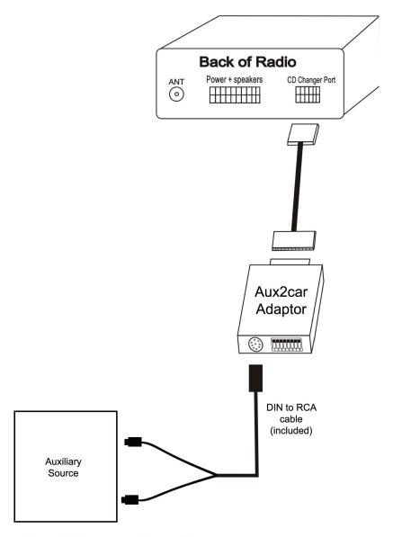
Connect Auxiliary source to female RCA input
