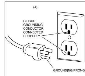
AN EXTENSION CORD MAY BE USED WITH CARE; HOWEVER, THE MARKED ELECTRICAL RATING SHOULD BE AT LEAST AS GREAT AS THE ELECTRICAL RATING OF THE APPLIANCE. Use only 3-wire extension cords which have 3-prong grounding-type plugs and 3-pole cord connectors that accept the plug from the appliance. The cord should be arranged so that it will not drape over the countertop or tabletop where it can be pulled on by
