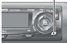
The face plate automatically closes after a lapse of 5 seconds while it is open.
