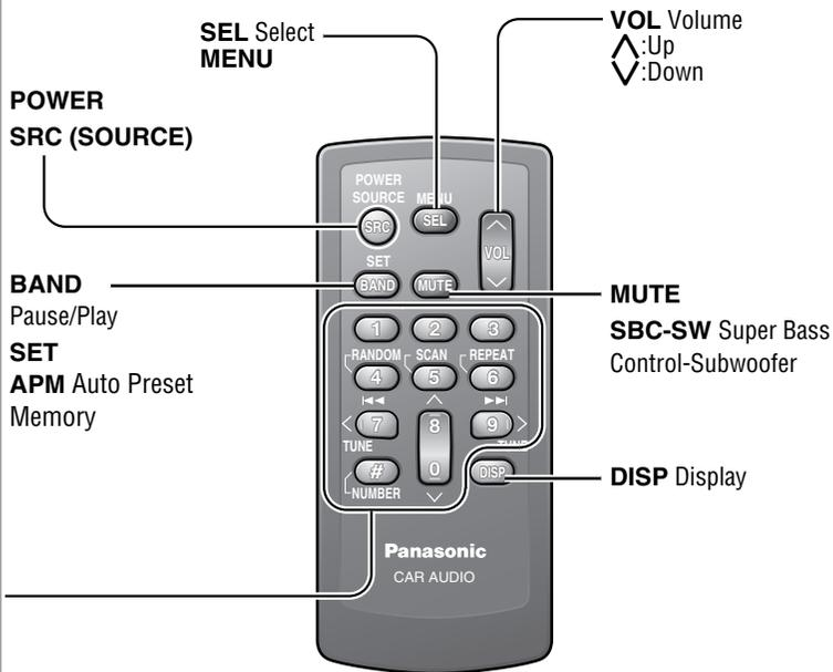
Although most of the functions of this unit are executable with both the main unit and remote control, the following functions are excluded.
