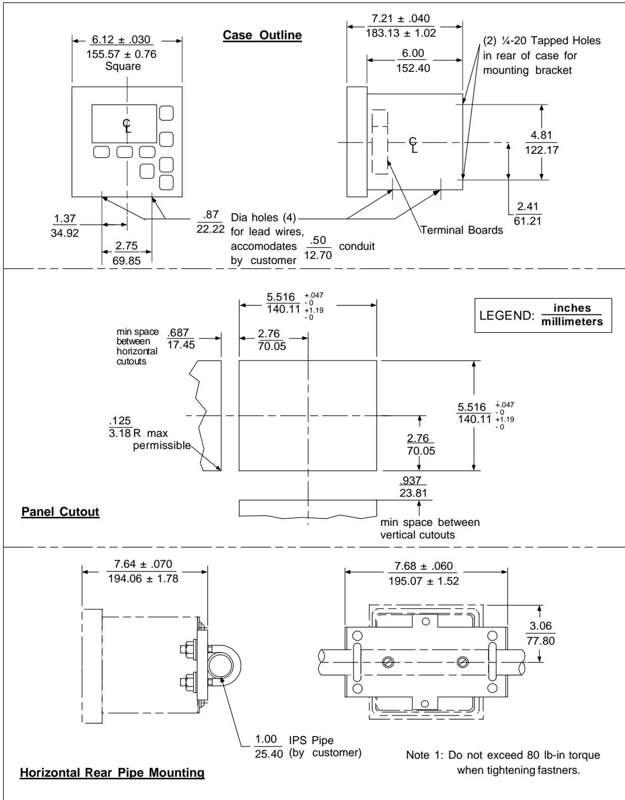
Figure 3-3-1 Mounting and Dimensions – Backlit Display Option
