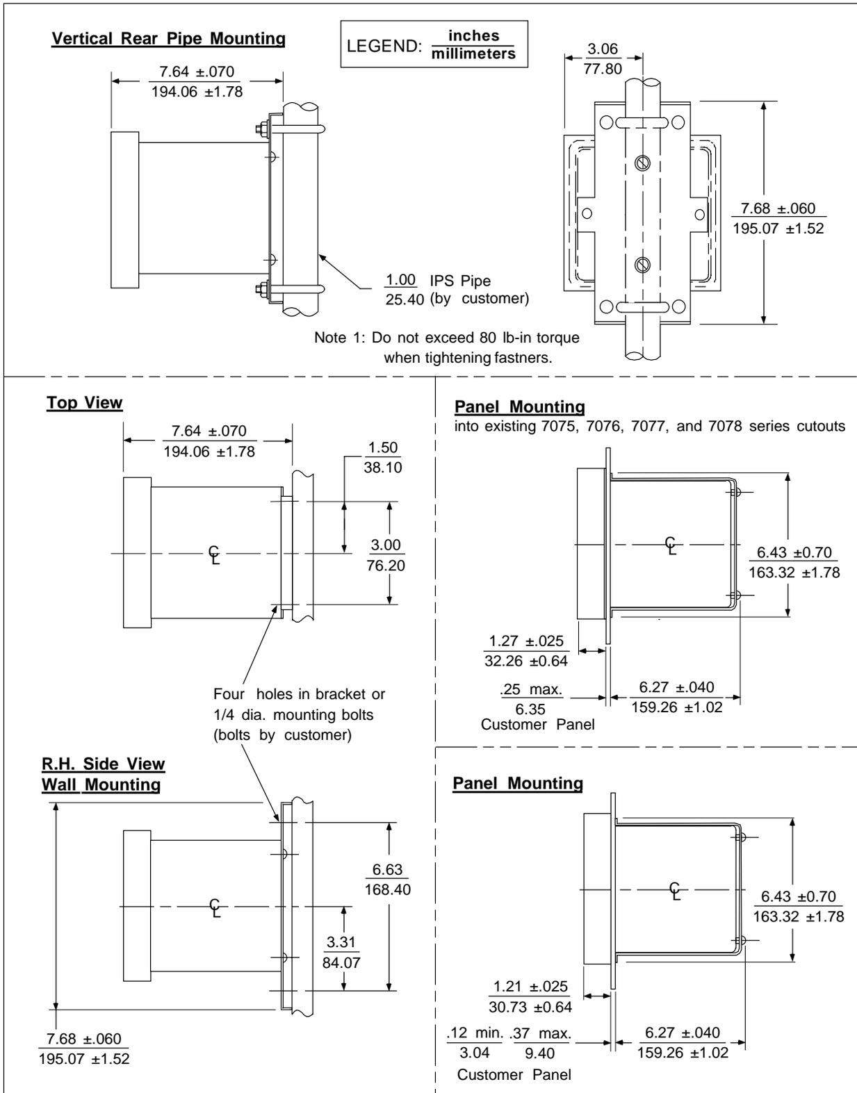
Figure 3-3-2 Mounting and Dimensions – Backlit Display Option
