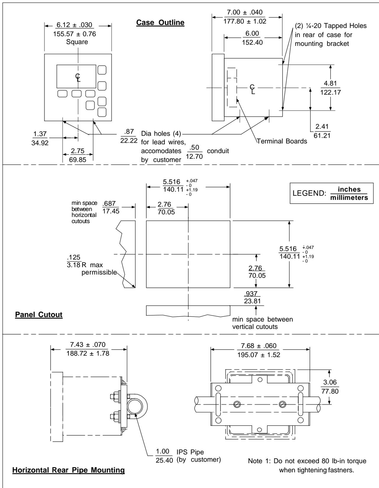
Figure 3-2-1 Mounting and Dimensions – Non-Backlit Display Option
