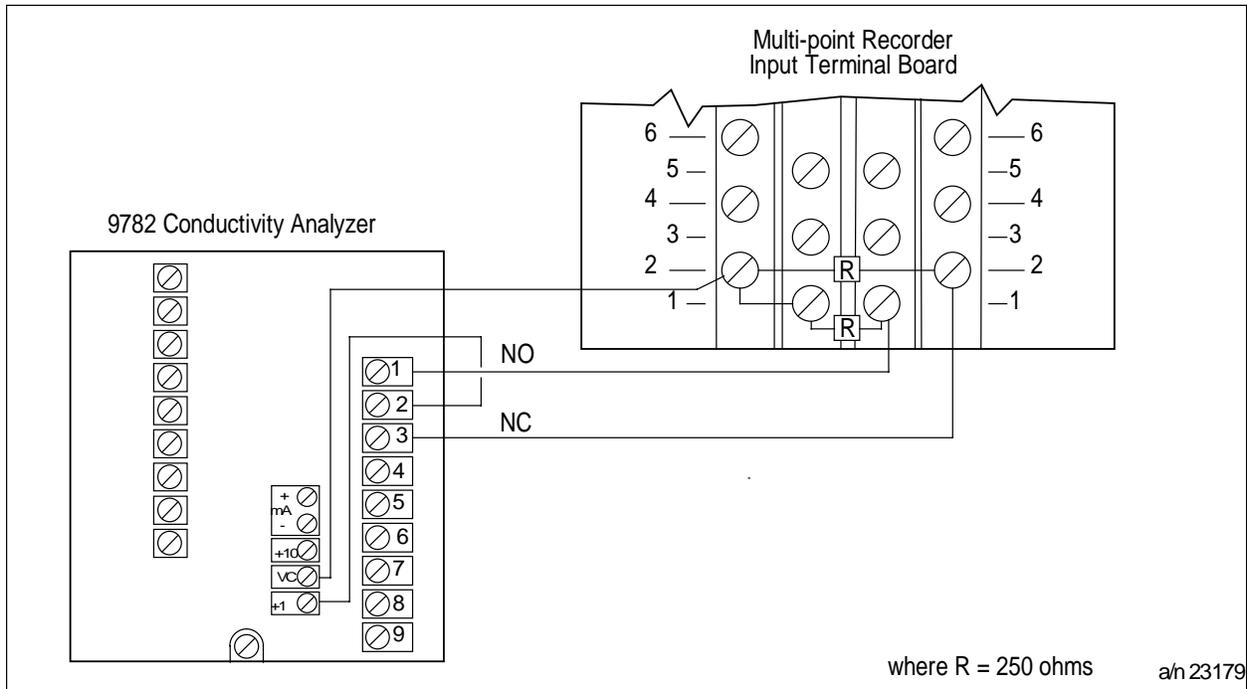
**Figure 6-3 Interconnections between 9782 and Recorder with Range Identification by Point Change**
