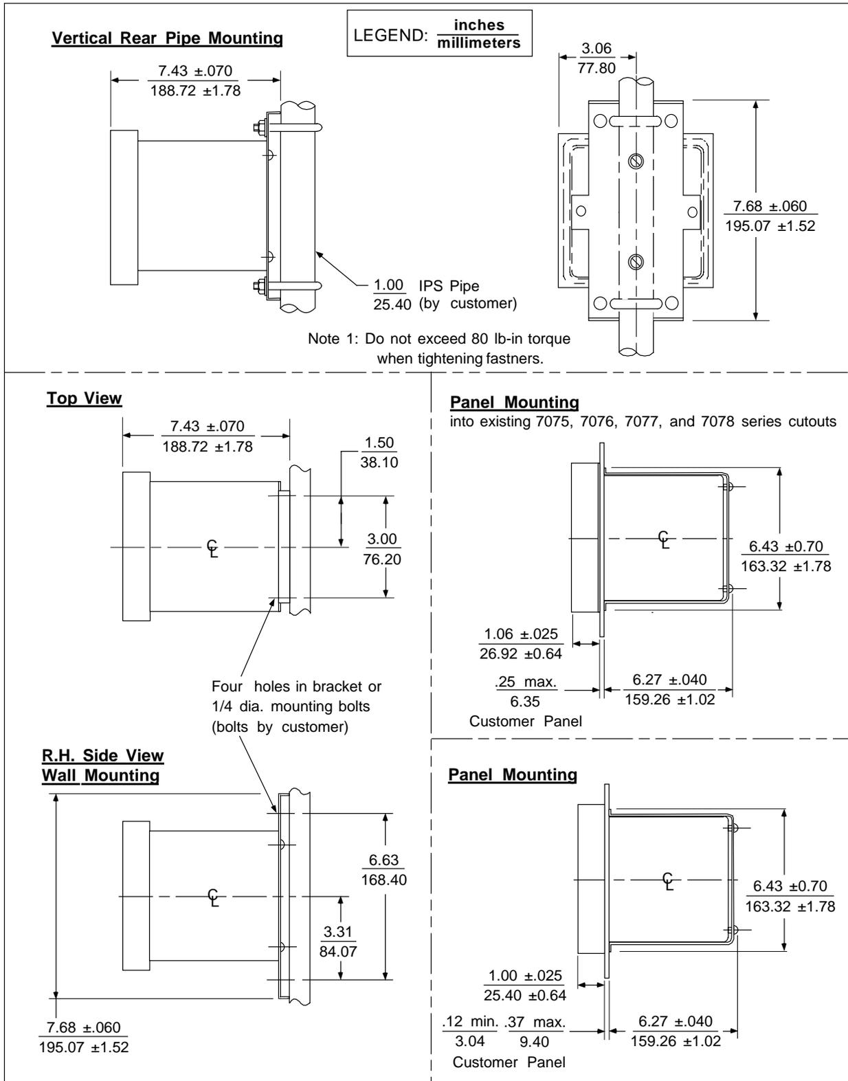
Figure 3-2-2 Mounting and Dimensions – Non-Backlit Display Option
