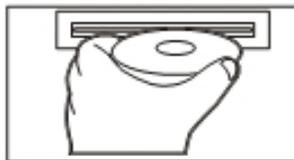
Note: If there is already a CD in the CD slot, do not try to insert a second CD, for this may damage the device.
