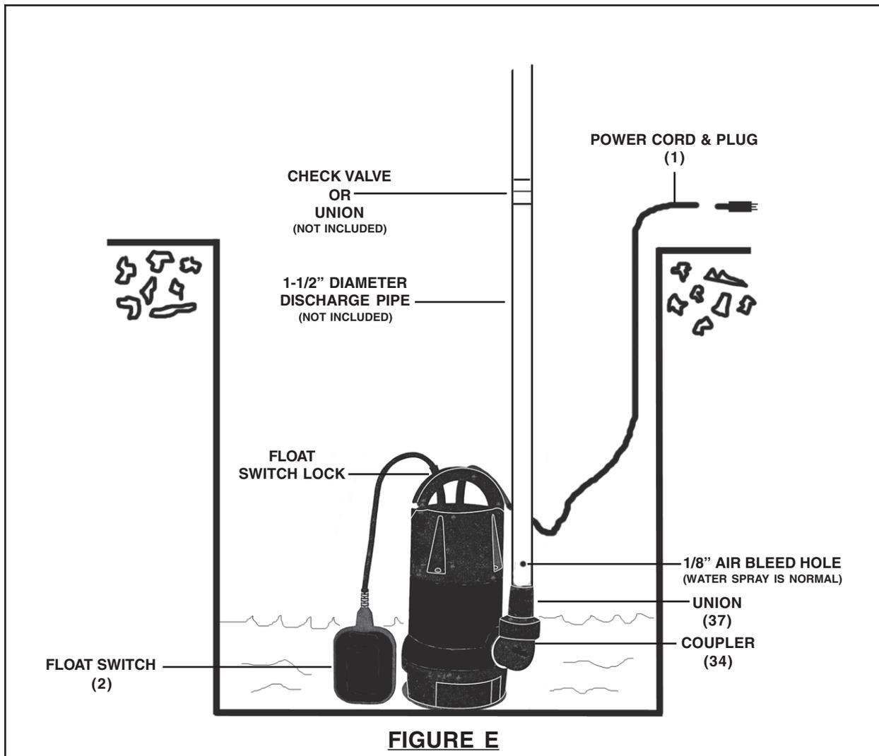
7. Carefully set the Pump in place. **Do not lower or raise the Pump by its Power Cord (1) or Discharge Pipe. (See Figure E.)**
