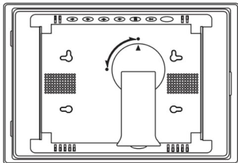
Your frame can also be wall-mounted. Use the slots on the back of the frame for either horizontal or vertical mounting.
