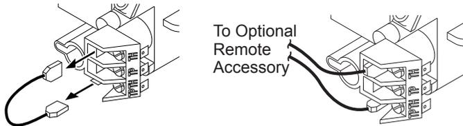
**Figure 37 - Disconnecting TH to TPTH Wire**
