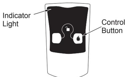
Figure 52 - On/Off Hand-Held Remote Control Unit HRC100
