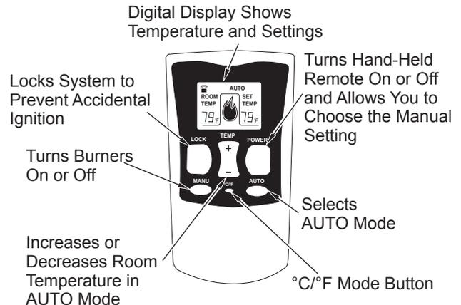
Figure 53 - Thermostat Hand-Held Remote Control Unit HRC200
