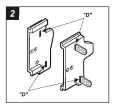
Slide *Mounting Tabs #3* into slots "D" on *Bracket Set #2*. The Mounting Tabs, Brackets and Bracket slots can be identified by the stamped letter on each component. *Skip to the Installation Instructions for ALL VEHICLES on Page #10*.
