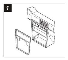
Disconnect the negative battery terminal to prevent an accidental short circuit. Unclip the climate control trim panel and remove (2) screws exposed. Remove (2) screws above the radio opening. Unclip the dash trim bezel, disconnect the wiring and remove the bezel. Remove (4) screws securing the factory head unit and disconnect the wiring.
