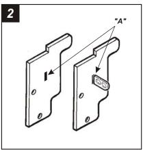
Slide Mounting Tabs #3 into slots "A" on Bracket Set #1. The Mounting Tabs, Brackets and Bracket slots can be identified by the stamped letter on each component. Skip to the Installation Instructions for ALL VEHICLES on Page #10.
