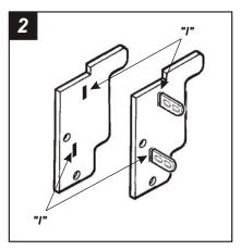
Slide *Mounting Tabs #3* into slots "I" on *Bracket Set #12*. The Mounting Tabs, Brackets and Bracket slots can be identified by the stamped letter on each component. *Skip to the Installation Instructions for ALL VEHICLES on Page #10*.
