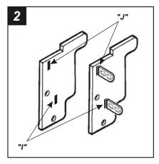
Slide Mounting Tabs #3 into slots "J" and "I" on Bracket Set #1. The Mounting Tabs. Brackets and Bracket slots can be identified by the stamped letter on each component. Skip to the Installation Instructions for ALL VEHICLES on Page #10.
