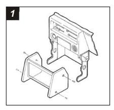
Disconnect the negative battery terminal to prevent an accidental short circuit. Remove (2) Phillips screws from each side of the radio trim bezel. Remove the bezel. Remove (4) screws securing the factory head unit and disconnect the wiring.
