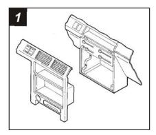
Disconnect the negative battery terminal to prevent an accidental short circuit. Remove (1) screw to the right of the ignition switch. Remove (1) screw above the left speaker. Unclip the dash trim bezel (some force may be required). Remove the screws securing the factory head unit and disconnect the wiring.
