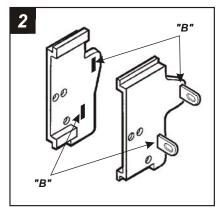
Slide *Mounting Tabs #3* and #8 into slots "B" on *Bracket Set #2*. The Mounting Tabs, Brackets and Bracket slots can be identified by the stamped letter on each component. Skip to the Installation Instructions for ALL VEHICLES on Page #10.
