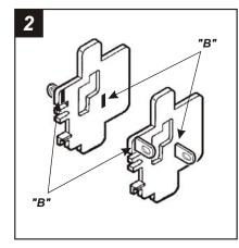
Slide **Mounting Tabs #3** and **#8** into slots **"B"** on **Bracket Set #12**. The Mounting Tabs, Brackets and Bracket slots can be identified by the stamped letter on each component. Skip to the Installation Instructions for ALL VEHICLES on Page #10
