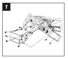
Disconnect the negative battery terminal to prevent an accidental short circuit. Remove (3) screws from the lower edge of the climate control panel. Remove (8) screws from the perimeter of the dash trim bezel. Pull out on the lower edge of the bezel and remove. Remove the screws securing the factory head unit and disconnect the wiring.
