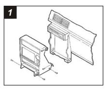
Disconnect the negative battery terminal to prevent an accidental short circuit. Remove (2) screws from the lower steering column panel and remove the panel. Remove (2) screws exposed on the dash trim bezel. Open the glove box and remove (2) screws exposed. Remove (2) screws from the ashtray cavity and (2) screws from the bracket. Remove (2) screws from each side of the dash trim bezel and unclip the bezel. Remove the screws securing the factory head unit and disconnect the wiring.
