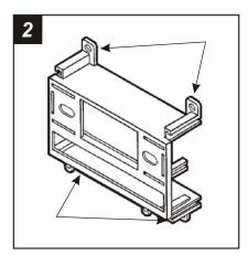
Locate the Mounting tabs on **Radio Housing #1.** (Brackets are NOT required for this vehicle). Skip to the Installation Instructions for ALL VEHICLES on Page
