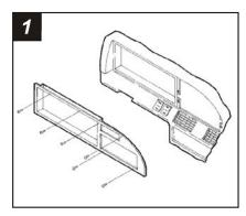
Disconnect the negative battery terminal to prevent an accidental short circuit. Remove (4) screws from the top edge of the dash trim bezel. Remove (2) screws below the radio opening. Remove (1) screw from the lower-left tab of the dash trim bezel (to the right of the a/c vent). Unclip the bezel. Remove the screws securing the factory head unit and disconnect the wiring.
