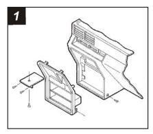
Disconnect the negative battery terminal to prevent an accidental short circuit. Remove the ashtray and (3) screws from the ashtray bracket. Remove (1) screw from each side of the dash console and unclip the dash trim bezel. Remove the screws securing the factory head unit and disconnect the wiring.
