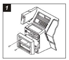
Disconnect the negative battery terminal to prevent an accidental short circuit. Remove (2) Phillips screws above the climate controls. Unclip the lower edge of the radio trim bezel and remove. Remove the screws securing the factory head unit and disconnect the wiring.
