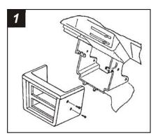
Disconnect the negative battery terminal to prevent an accidental short circuit. Remove (2) screws from each side of the dash trim bezel and remove the bezel. Remove (4) screws securing the upper radio dummy cover to the bezel and remove.
