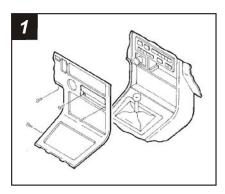
Disconnect the negative battery terminal to prevent an accidental short circuit. Remove the ashtray and (2) screws from the ashtray cavity. Remove (1) screw to the right of the steering column and (1) screw to the left of the gear shifter. Remove the screws securing the factory head unit and disconnect the wiring.
