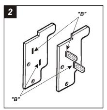
Slide Mounting Tabs #3 into slots "B" on Bracket Set #1. The Mounting Tabs, Brackets and Bracket slots can be identified by the stamped letter on each component. Skip to the Installation Instructions for ALL VEHICLES on Page #10.
