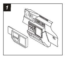
Disconnect the negative battery terminal to prevent an accidental short circuit. Remove (3) Phillips screws above the climate controls. Remove (2) Phillips screws from the left side of the dash trim bezel and remove the bezel. Remove the screws securing the factory head unit and disconnect the wiring.
