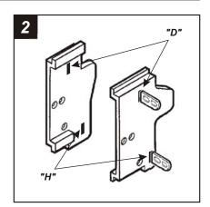
Slide *Mounting Tabs #3* into slots "H" and "D" on *Bracket Set #2*. The Mounting Tabs, Brackets and Bracket slots can be identified by the stamped letter on each component. Skip to the Installation Instructions for ALL VEHICLES on Page #10.
