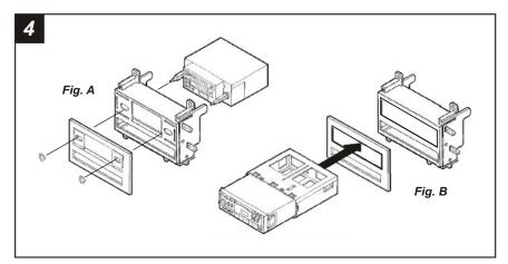
**2-SHAFT HEAD UNITS:** Snap the Faceplate onto the front of the Radio Housing. (For applications using *Faceplate #2*, cut and remove the bottom portion of the Faceplate). Slide the aftermarket head unit into the kit and secure with shaft nuts. (see Fig. A)
