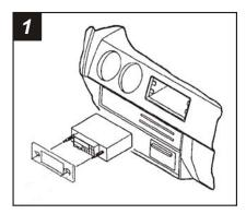
Disconnect the negative battery terminal to prevent an accidental short circuit. Remove (4) Phillips screws securing the factory head unit and disconnect the wiring.
