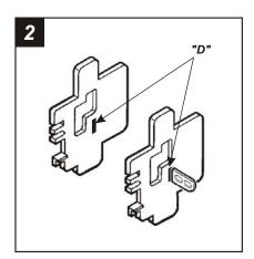
Slide Mounting Tabs #3 into slots "D" on Bracket Set #12. The Mounting Tabs, Brackets and Bracket slots can be identified by the stamped letter on each component. Skip to the Installation Instructions for ALL VEHICLES on Page #10.
