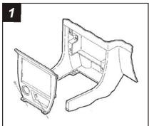
Disconnect the negative battery terminal to prevent an accidental short circuit. Prv up on the gear shifter trim panel and remove the panel. Remove (2) screws exposed on the bottom edge of the radio trim bezel. Unclip the bezel, and disconnect the ashtray and cigarette lighter wiring. Remove the screws securing the factory head unit and disconnect the wiring.
