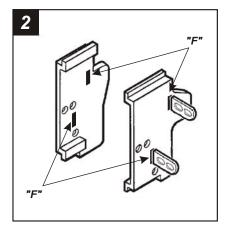
Slide *Mounting Tabs #3* into slots *"F"* on *Bracket Set #2.* The Mounting Tabs, Brackets and Bracket slots can be identified by the stamped letter on each component. *Skip to the Installation Instructions for ALL VEHICLES on Page #10.*
