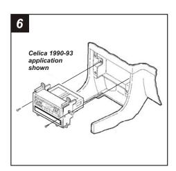
Re-connect the battery terminal and test the unit for proper operation. Mount the head unit/kit assembly to the sub-dash with those screws previously removed in step #1. (It may be necessary to trim the ends of the Mounting Tabs to provide proper clearance).
