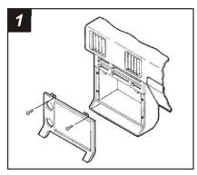
Disconnect the negative battery terminal to prevent an accidental short circuit. Remove the ashtray and the climate control knobs. Remove (3) flat-head screws from the climate control panel and remove the panel. Remove (2) Phillips screws from the top edge of the radio trim bezel. Remove (4) Phillips screws from the base of the radio trim bezel and remove the bezel. Remove (4) Phillips screws from the factory head unit and disconnect the wiring.
