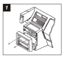
Disconnect the negative battery terminal to prevent an accidental short circuit. Remove (2) screws from the top of the dash trim bezel and remove the bezel. Remove (4) screws from the factory head unit (or coin tray dummy panel) and disconnect the wiring.
