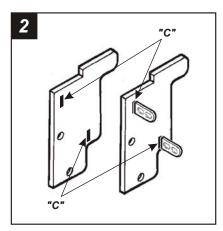
Slide *Mounting Tabs #3* into slots *"C"* on *Bracket Set #1*. The Mounting Tabs, Brackets and Bracket slots can be identified by the stamped letter on each component. *Skip to the Installation Instructions for ALL VEHICLES on Page #10*.
