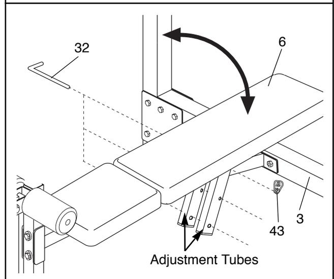
**WARNING: When adjusting the position of the seat, make sure that the adjustment pin is inserted through both adjustment tubes before beginning any exercise.**
