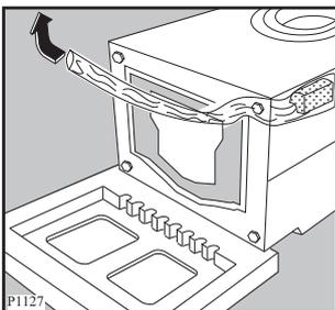
Remove the polystyrene base. Set the machine upright and unscrew the remaining rear screw. Slide out the relevant pin. Fill all the holes with the plastic plugs supplied with the instruction booklet.
