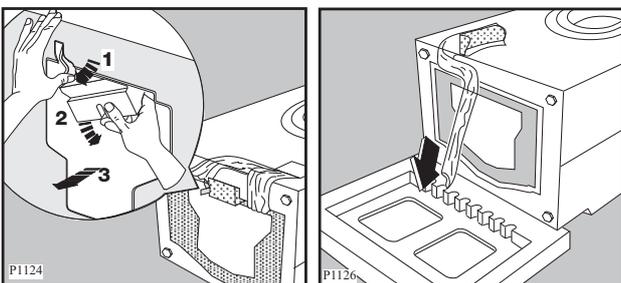
Repeat the operation for the right polythene bag, removing it towards the left and then upwards.
