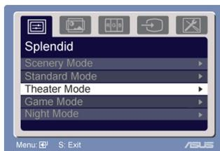
2. Press ▼ and ▲ to navigate through the functions. Highlight and activate the desired function by pressing the MENU button. If the function selected has a sub-menu, press ▼ and ▲ again to navigate through the sub-menu functions. Highlight and activate the desired sub-menu function by pressing the MENU button.
