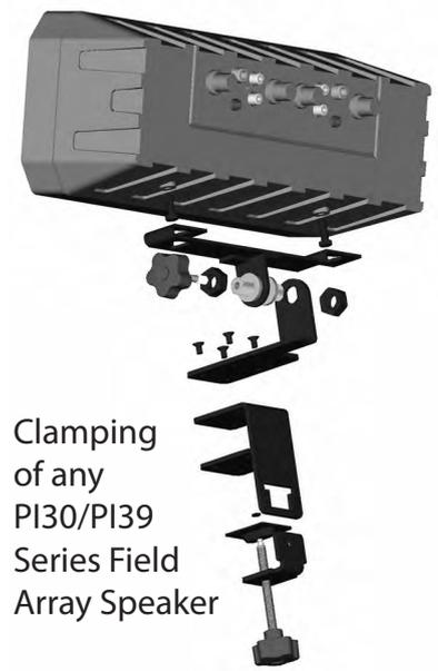
Clamping of any PI30/PI39 Series Field Array Speaker
