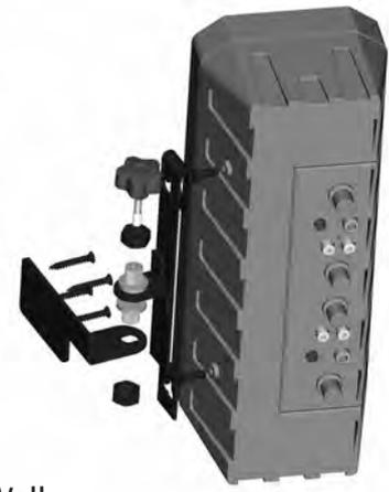
Wall Mounting of any PI30/PI39 Series Field Array Speaker
