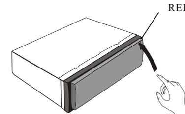
When the front panel was turned down to a position of 45°, hold and slide the front panel to left, and then pull it out.
