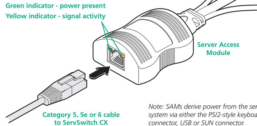
*Note: SAMs derive power from the server system via either the PS/2-style keyboard connector, USB or SUN connector.*
