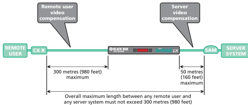
*Note: For installations where both servers and remote users require video compensation, always ensure that the servers are compensated first.*
