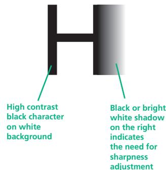
*Note: The Word processor method is accurate and quick. However, for the very finest video compensation, use the latest "skew" test pattern program which shows both the skew pattern and a section of mixed size Hs (black on white and white on black).*
