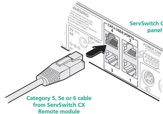
*Note: The ServSwitch CX model shown here is a non-IP version. The IP-version provides only remote user ports 3 and 4.*
