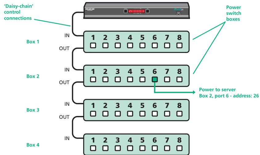
The power ports are connected to the power inputs of each server system and the power switch box(es) are then connected to a mains power supply.
