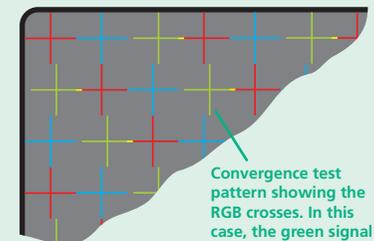
The screen will show a series of fine red, green and blue crosses which should all be in line, vertically and horizontally. Skew affects the horizontal placement of the colours and using this pattern it is much easier to discover which, if any, colours are being adversely affected by the cable link.
