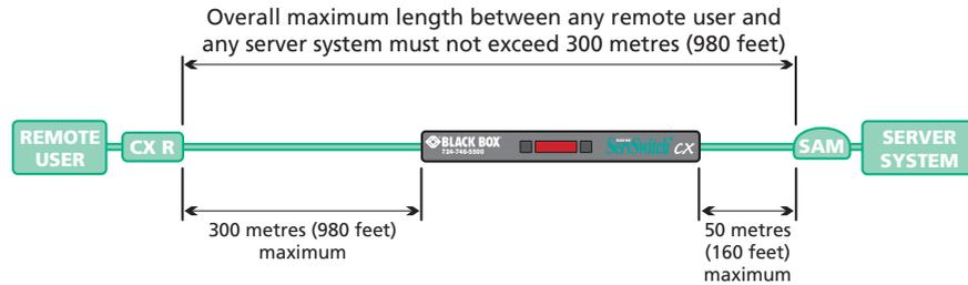
In situations where any server system will be placed a significant distance from the ServSwitch CX unit, ensure that the distance to any remote user is similar less than 300 metres (980 feet).
