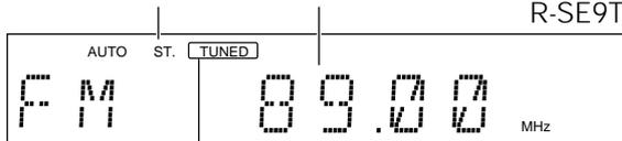
The "TUNED" indicator lights when a station is received.
