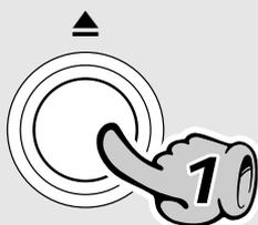
The tray opens when the key is pressed and closes when the key is pressed again.
