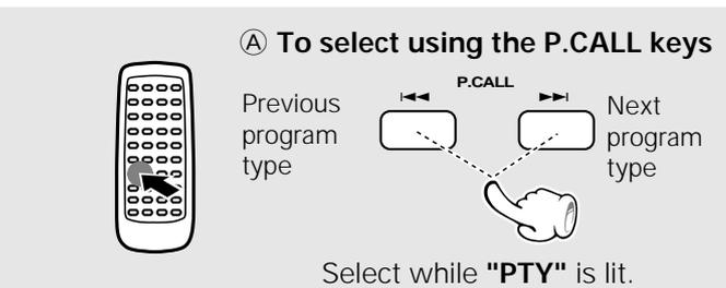
The P.CALL keys let you select from all 29 program types in the order shown at right. Press the key and release it when the desired type is displayed.
