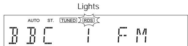
The "RDS" indicator lights up when an RDS broadcast (signal) is received.
