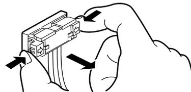
While pushing the two sides of connector in, pull it straight out.
