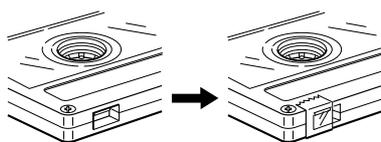
Apply tape only to the position where the tab has been removed.
