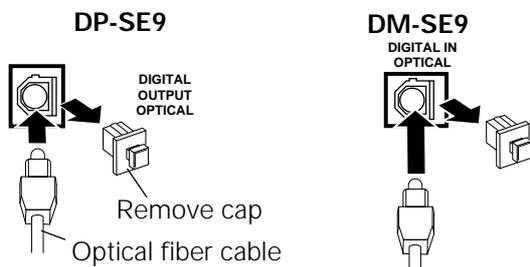
This is used for digital connections. Digital transmission permits recording without loss of the high CD sound quality.
