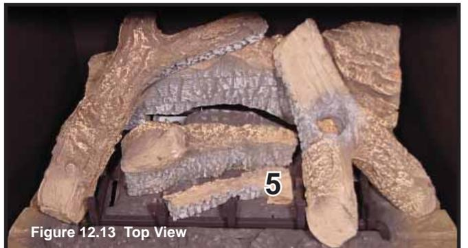
**STEP 7. Log #5 (SRV2103-111):** Place log #5 in front of log #3 the notch in the bottom of this log rests over the center tine on the grate. The log shouldn't cover any ports.
