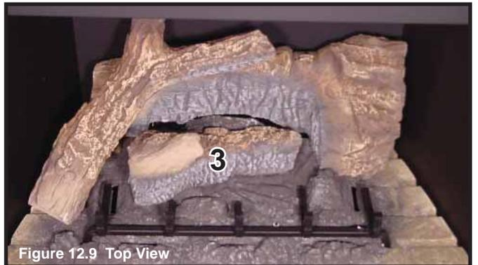
**STEP 5. Log #3 (SRV2103-110):** Place log #3 on top of the burner surface in front of the hump. The bottom of the log has a square groove cut through it. The groove sits over the second grate tine from the left. Slide it back against the hump.
