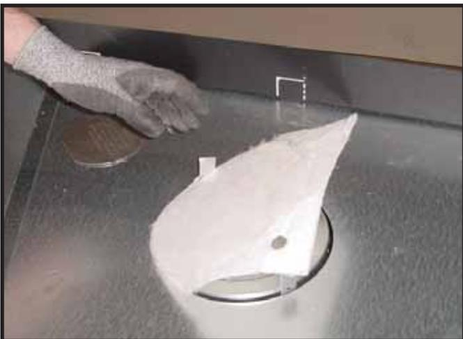
**Figure 7.3** Remove the white gasket material covering the seal cap.
