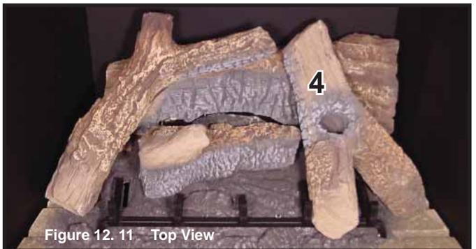
**STEP 6. Log #4 (SRV2103-109):** Place log #4 on top of the right side of log #1. The bottom of this log has a slot in it that goes over the tab molded into the top of log #1. The other end of the log rests on the grate, against the second tine from the right.
